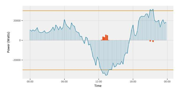
Between 12:30 and 13:45, generation causes too much feed in and at both 21:00 and 21:30, consumption is too high. Both situations will cause an overload if no measures are taken so the DSO requests flexibility using a *FlexRequest* to reduce the load on the grid. The amount of flexibility needed is depicted in red<sup>1</sup>.
