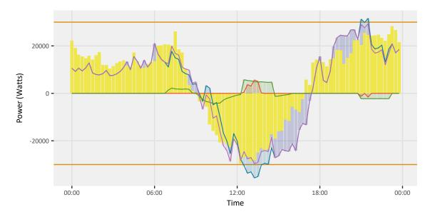
The actual values differs from the prognosed values. Although the difference between actual values and the values in the final D-prognosis are substantial for certain PTUs, the offered flexibility can be realized by the aggregator, even although the algorithms used by the aggregator are very basic.
