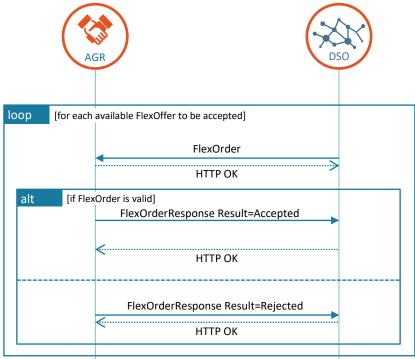
Figure 3-10: Exchange of FlexOrder
