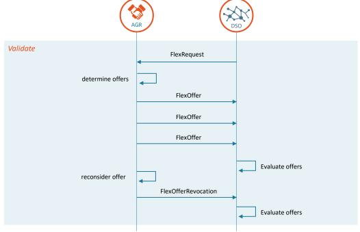
Figure 2-6: AGR may send multiple FlexOffers on the same request, and open FlexOffers, which are not yet ordered may be revoked by the AGR.
