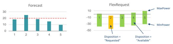
Figure 2-8: Example forecast for a Congestion point, leading to an example FlexRequest, both displayed in graphs
