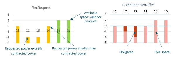
Figure 4-3: Example FlexRequest and requirements of FlexOffer, displayed in graphs
