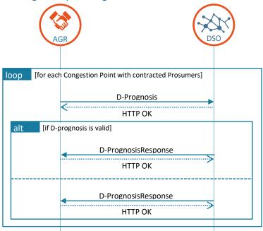
Figure 3-6: Exchange of D-prognoses
