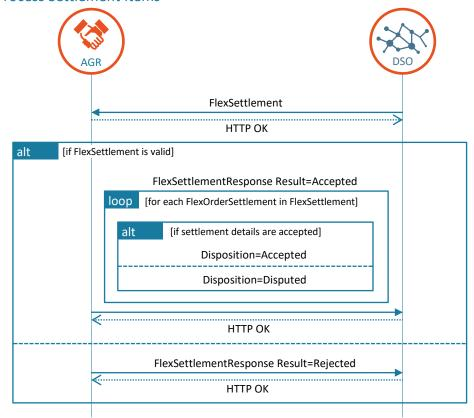
Figure 3-11: Transmission of settlement including acceptance process per settlement item
