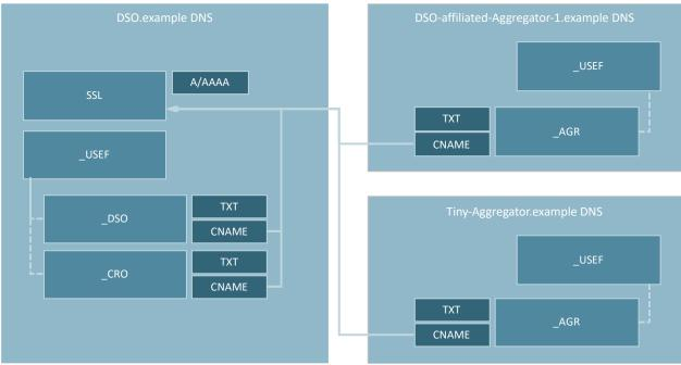
Figure 4-5 Example of the DNS relationships between a single USEF endpoint and multiple zones
