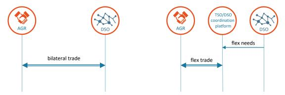
USEF assumes that a DSO or TSO can freely and independently trade flexibility with AGRs. Any potential goal conflicts can be settled through the market mechanism. Alternatively, TSO and DSO requests can be aligned, resulting in a TSO/DSO coordination platform where TSOs and DSOs coordinate the tendering, trading, activation and/or settlement of flexibility for their own purposes (i.e. ancillary services). See [2] for a discussion on this topic.
